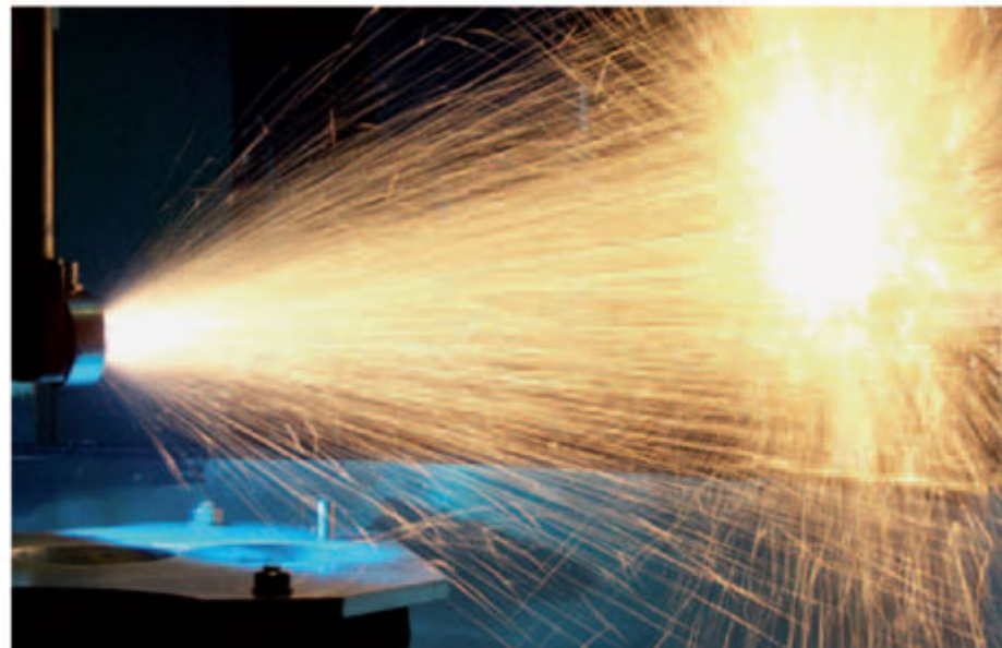
3 The TWAS overlay process for creating ferrous overlays in aluminum crankcase housings
